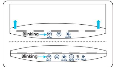
Open the flip-up lid and press the airflow speed touch button. When the Wi-Fi symbol starts to blink, the air purifier can be paired with the Blueair Friend mobile app.
