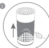
Remove the pre-filter from the unit's metal frame.
