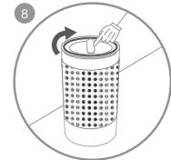
Replace the bottom by gently pushing it down and simultaneously rotating it clockwise to secure it back into the bayonet lock.
