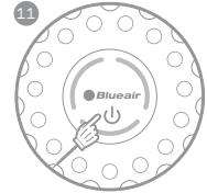
Press the touch button for a duration of 5 seconds to reset the filter replacement timer. This lets JOY S know that you have changed the filter. The indicator light flashes 3 times, and then changes from red to white.
