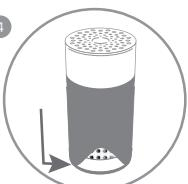
Pull the bottom elastic end of the pre-filter over the bottom edge of the air purifier.
