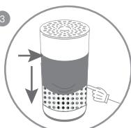
Refit the pre-filter back onto the unit's metal frame by guiding the top elastic end into the slot between the top cylinder and the metal frame.
