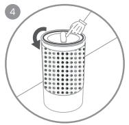
Carefully place the unit upside down on a flat surface and open the bottom by rotating it counter-clockwise whilst holding the unit.
