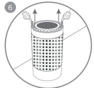
Grip the handles on the main filter and pull upwards to remove the main filter from the unit.
