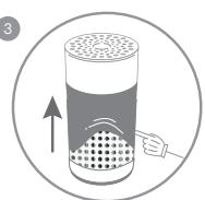
Remove the pre-filter from the unit's metal frame.
